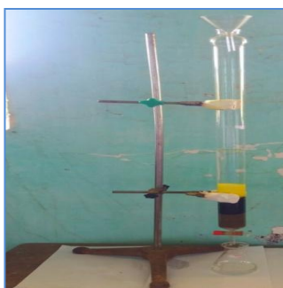
Figure 1 Treatment of water sample by column filtration process
